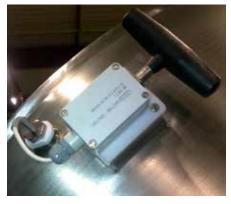
Radio frequency probe for total control of the product temperature
